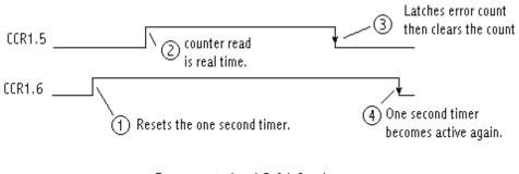
Transparent when 1.5 & 1.6 = 1 Latches & clears when 1.6 = 1 and 1.5  $\checkmark$
